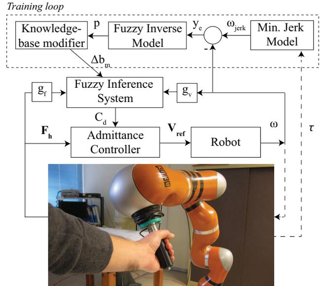
Fig. 1. Fuzzy Model Reference learning of variable admittance control for human-robot cooperation in rotational motion.
