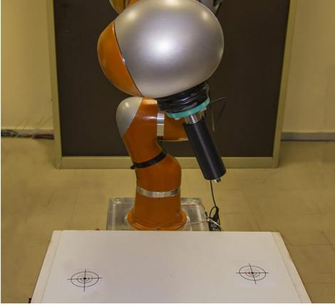
Fig. 3. Experimental setup for human-robot cooperation in a rotational motion between to targets.
