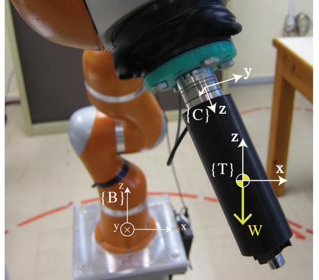
Fig. 2. Tool weight compensation from the 6DOF force/torque sensor at the robot's end-effector.
