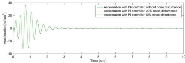
Fig. 9. PI-based vibration control of the acceleration response at the free end of the beam.
