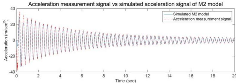
**Fig. 6.** Actual acceleration response signal at the free-end of the beam and its ARX(4,4) model based simulation.
