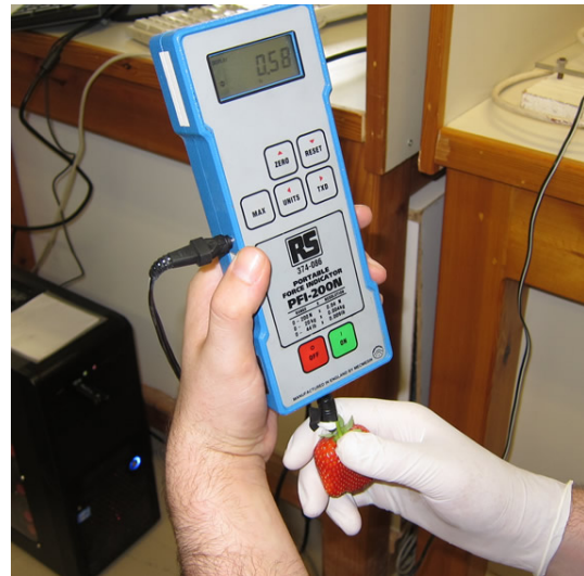
Fig. 3: Measuring detachment force with a portable force sensor
